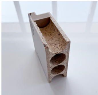
High pressure particle core with acoustic transmission reduction holes in door leafs
